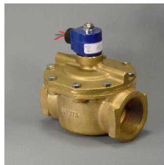
S21 Piloted Diaphragm 1" to 2" Brass or 316 Stainless Steel 10 to 150 psi Water 10 to 150 psi Steam
