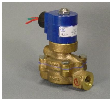
S21..T2 Piloted Diaphragm 3/8", 1/2", 3/4" Brass 10 to 150 psi Water 10 to 150 psi Steam
