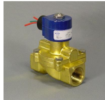
S21..T4 Piloted Diaphragm 3/8", 1/2", 3/4" Brass 10 to 250 psi Water 10 to 100 psi Steam
