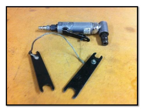
**Note:** Operating this type of pneumatic angle grinder will quickly use a large volume of air from you compressor tank. Smaller air compressors (30 gallons or less) will run almost consistently when using this tool at high speeds for prolonged periods of time.
