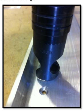
I solved this by grinding away part of countersink Microstop housing. This Microstop has a plastic screwin insert which I removed for this task. I can still screw the plastic ring in for countersinking where clearance is not a problem.
