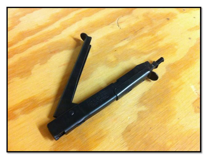
This tool is incredibly handy for removing small amounts of thin (up to .040" approx.) aluminum in tight areas when making parts or repairing structure. Included below are some photos of the nibbler in action on .032" T6 aluminum.
