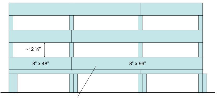
SUPPORT STRIPS – 1 SHEET OF 4'X8' 3/8" CHIP BOARD RIP INTO 6 STRIPS OF 8" WIDE, CUT 2 STRIPS TO 48" LONG LAY OUT STRIPS AS SHOWN TO FORM 12' WIDE SUPPORT FRAME ATTACH WITH 2 OF #6 X 1 5/8 DRYWALL SCREW AT EACH FRAME CROSSING.
