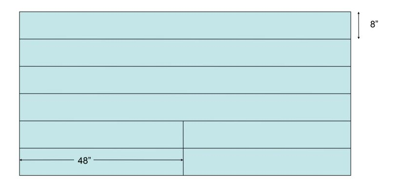
PLYWOOD SHEET CUT LAYOUT. LAST STRIP WILL BE NARROW BY CUMULATIVE WIDTH OF SAW KERF.
