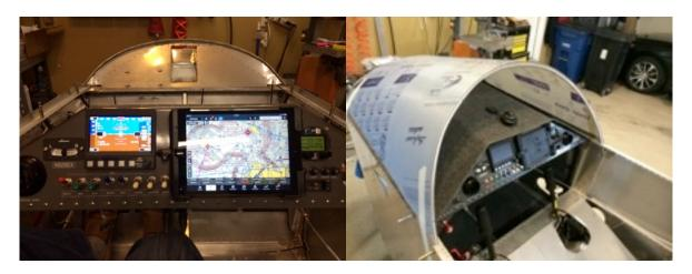
After finishing the panel I have completed the fuel system and permanently installed the fuel tank, glare shield and most recently finished the wind screen. That was a real challenge to bend and fit a flat piece of Lexan to a complex curve shape.
