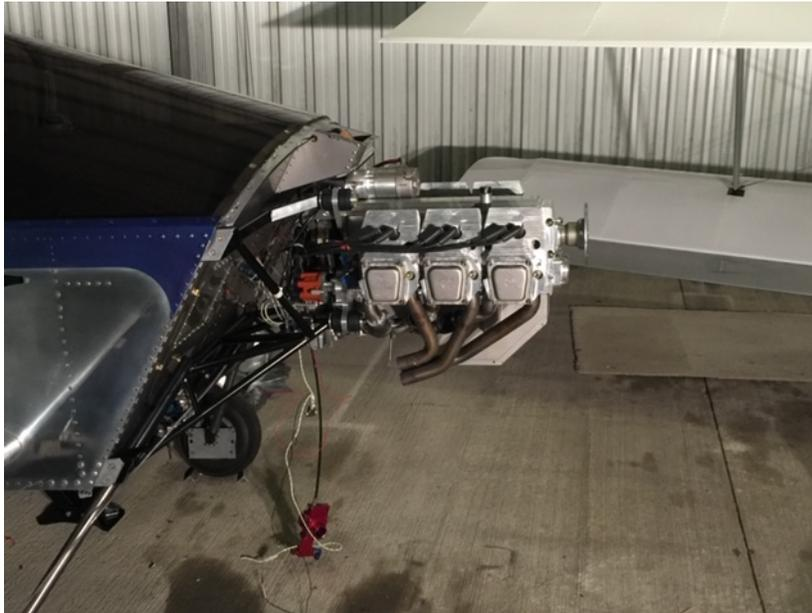
*New Jabiru engine mount and freshly overhauled Jabiru 3300 just installed*
