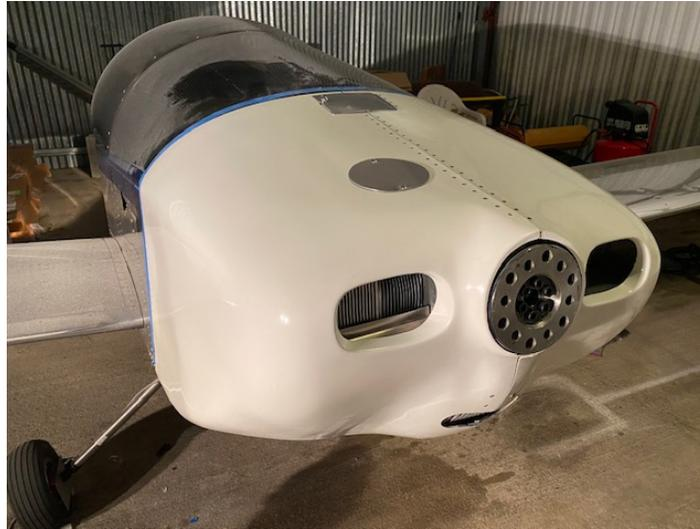
*New cowling and cooling baffles being fitted*
