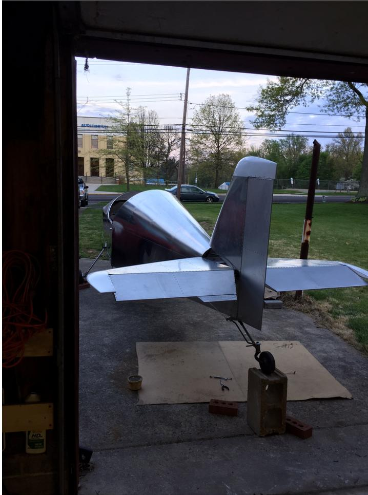
Differential cable brakes and modified full swivel Scott tail wheel. Standard canopy with bonded sides (no rivets), also Exterior canopy handle to open it.
