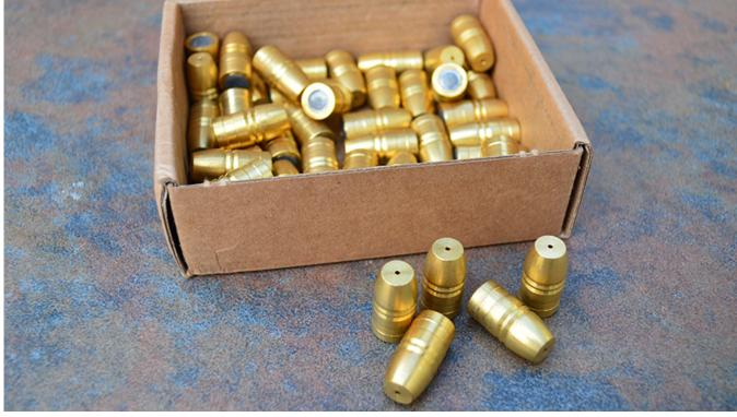
The Kodiak Punch bullet by Rintoul Enterprises is a no-compromise flat-nosed brass bullet with a lead insert for additional weight. In .50 caliber, this bullet weighs 420 grains and brings deep, straight-line penetration to the party. My loads were pushing this bullet right around 1400 fps.
