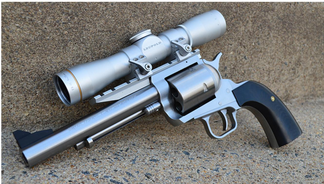
*A nod to the genius of Dick Casull. The .444 was replaced by this BFR in .454 Casull sporting a 6 ½-inch barrel. I equipped it with the same optic as the .444 Marlin version, a fixed 4X Leupold scope with the company's Quick Release rings.*
