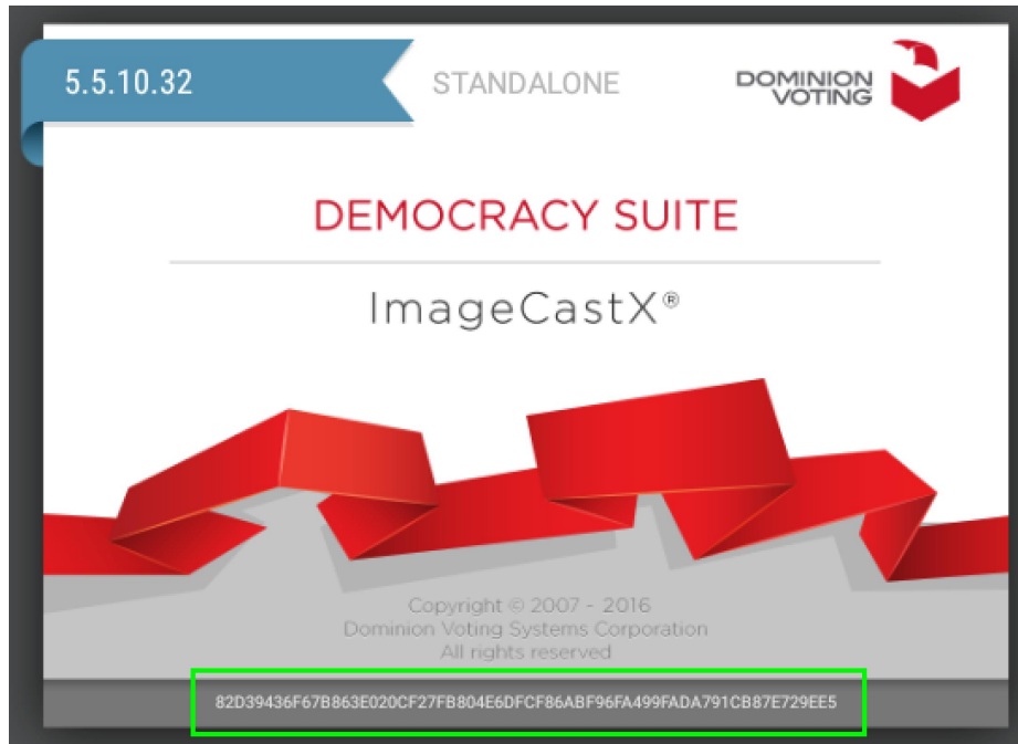
Figure 8: Defeating Hash Validation. The ICX App displays the SHA-256 hash of its APK on the screen, as shown here. However, this behavior is controlled by the app itself, so a maliciously modified app can simply show the expected hash value instead of its real one, thereby avoiding detection.
