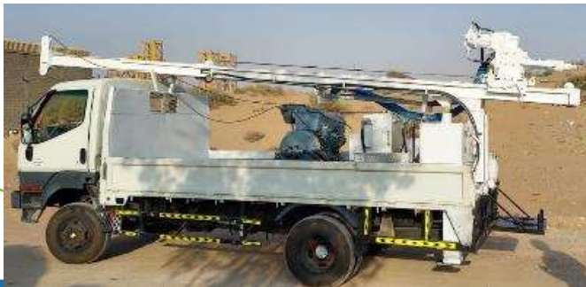
TRUCK MOUNTED GEOTECHNICAL ROTARY DRILLING RIG
