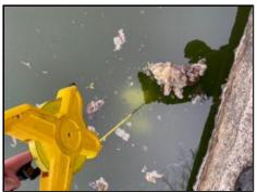
Figure 28: Secchi depth being measured at the Pond
