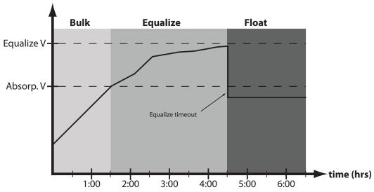
Figure 4-6. Equalize timeout charging profile
