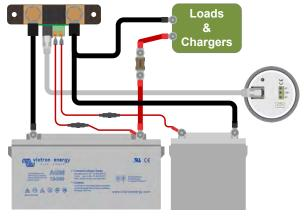
Battery monitor with auxiliary second battery monitoring.
