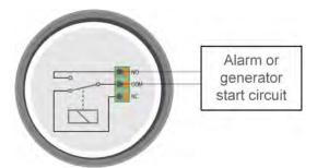
The internal wiring diagram of the battery monitor with the relay in a de-energised state connected to an external alarm or generator start circuit.
