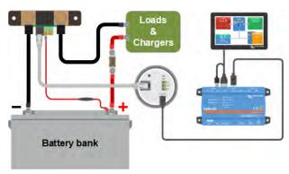
Example of a battery monitor connecting to a GX device.
