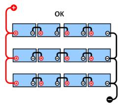
**GOOD:** The midpoints are not connected and without busbars or midpint monitoring.
