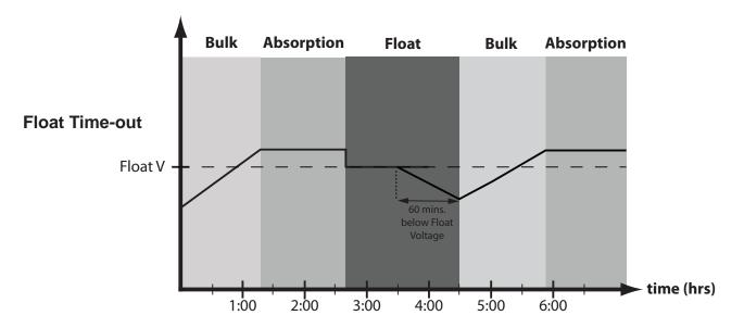
Figure 4-4. Float exit time-out charging profile
