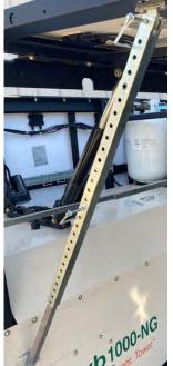
**Tele-Struts** - Used to stabilize solar wings during high winds, with use of Tele-tabs and pins. Included in units that have the high-wind package.
