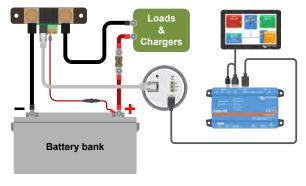
The battery monitor is connected to a Cerbo GX and a GX Touch screen.
