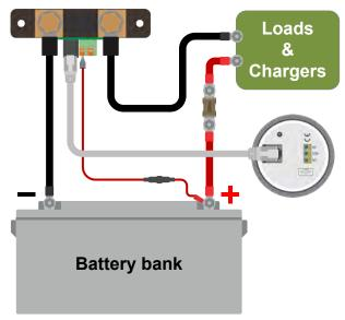
Basic battery monitor installation.
