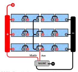
**GOOD:** The midpoints are connected, busbars are used and with midpoint monitoring.
