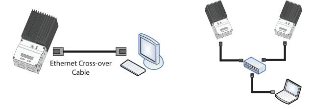
Figure 5-3. Ethernet network diagrams.
