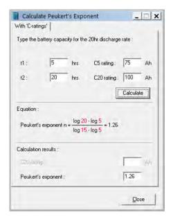
Please note that the Peukert exponent is no more than a rough approximation of reality. In case of very high currents, the battery will give even less capacity than predicted by a fixed exponent. We do not recommend changing the default value in the battery monitor, except in the case of lithium batteries.
