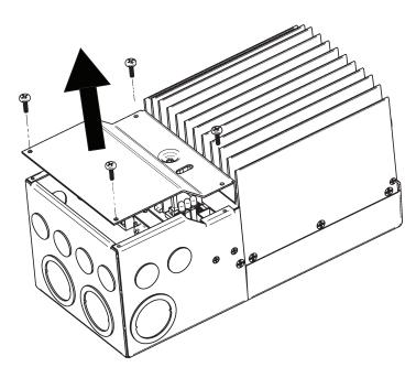
Figure 3-1. Remove the wiring box cover.
