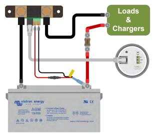
Battery monitor with auxiliary temperature sensing.
