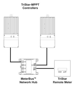
Figure 5-1. An example MeterBus network.
