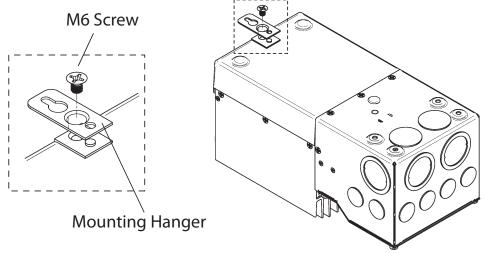
Figure 3-2. Attaching the mounting hanger
