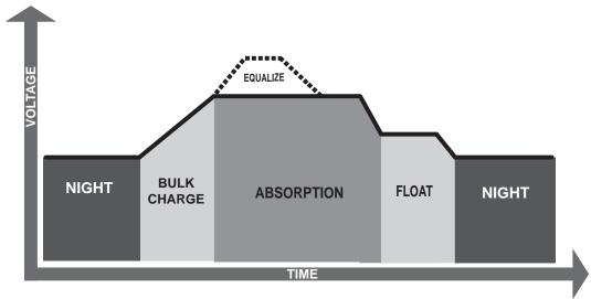
Figure 4-2. TriStar MPPT 150V Charging Algorithm
