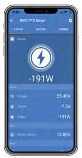
VictronConnect app status screen of a battery monitor running in DC monitor mode.
