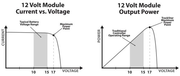
Figure 4-1. Nominal 12 Volt Solar Module I-V curve and output power graph.
