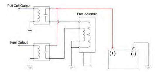
**Pull Coil Wiring Example**
