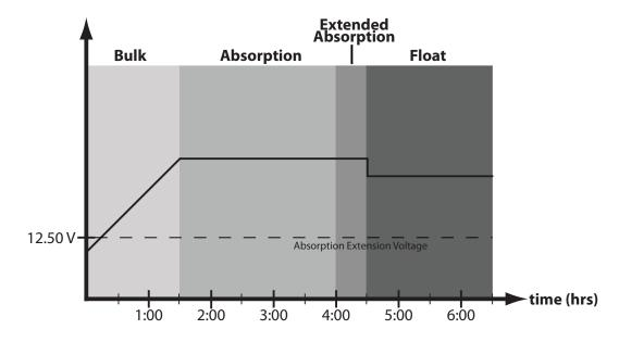
Figure 4-3. Absorption extension charging profile.
