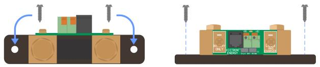
Top view shunt indicating mounting holes and side view shunt indicating the mounting method.
