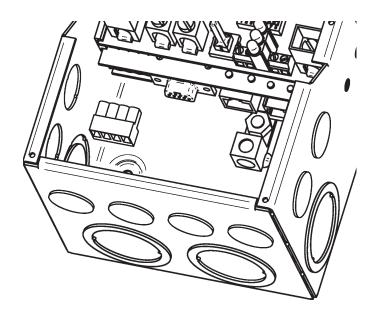
Figure 3-6. Removing the RS-485 socket connector
