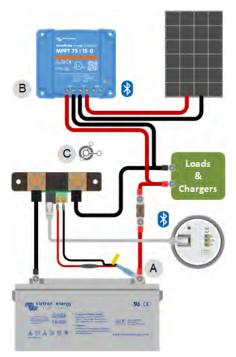
Example of a system containing a battery monitor with a temperature sensor and a solar charger, both using the VE.Smart networking.
