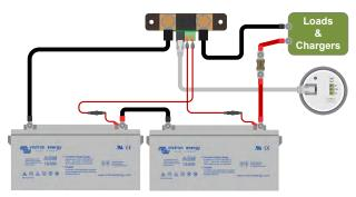
Battery monitor with auxiliary midpoint monitoring.
