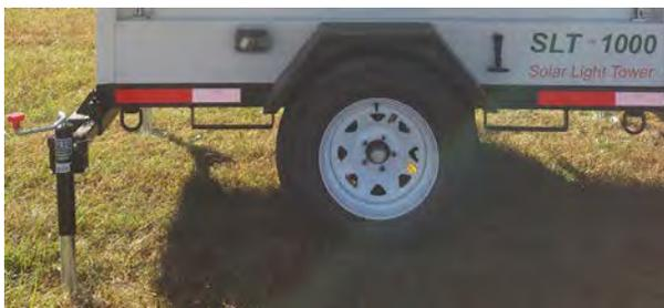
**D-ring Tie-Down Points**- Used to secure tower with straps / chains in order to apply equal force to both ends of the light towers if transported via a flat-bed truck or trailer while in tow. Locations vary by model.
