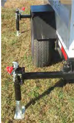
**Outriggers/Jack Stands** - to level unit and support the raised light tower mast. Deploy outriggers/jacks for stability. Located at the front (optional), rear and tongue of the trailer to provide stability while light tower is deployed.
