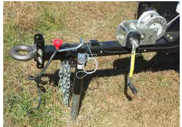
**Light / Brake Quick Connects**- 7 pin or 4 pin Quick connects attach wiring of trailer lights and brakes to towing vehicle.
