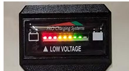
The operator sees the current charge levels in increments to maximize battery life, it is best to limit your discharge rate to no lower than 30% of the capacity of the battery bank and to fully charge the batteries on a routine basis. This charge can be achieved by either or a combination of solar gain or with an on-board backup electric (AC) battery charger.
