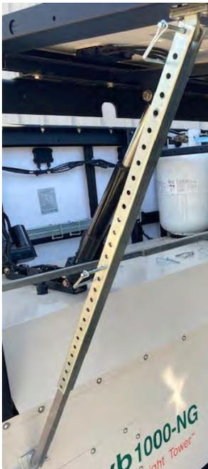
**Tele-Struts** - Used to stabilize solar wings during high winds, with use of Tele-tabs and pins. Included in units that have the high-wind package.
