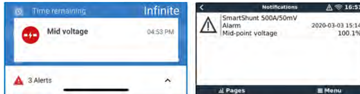
Left: alarm displayed on the VictronConnect app. Right: alarm displayed on a GX device.
