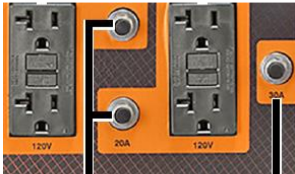
(2) 20Amp 1 P Push button Breakers
