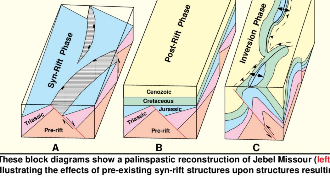
B) Deposition of Late Cretaceous and Cenozoic post-rift sedimentary rocks. fold with forelimb breakthrough. These folds have the opposite vergence resulting in the transport of thicker syn-rift strata from the hanging wall over thinner syn-rift strata from the footwall.
