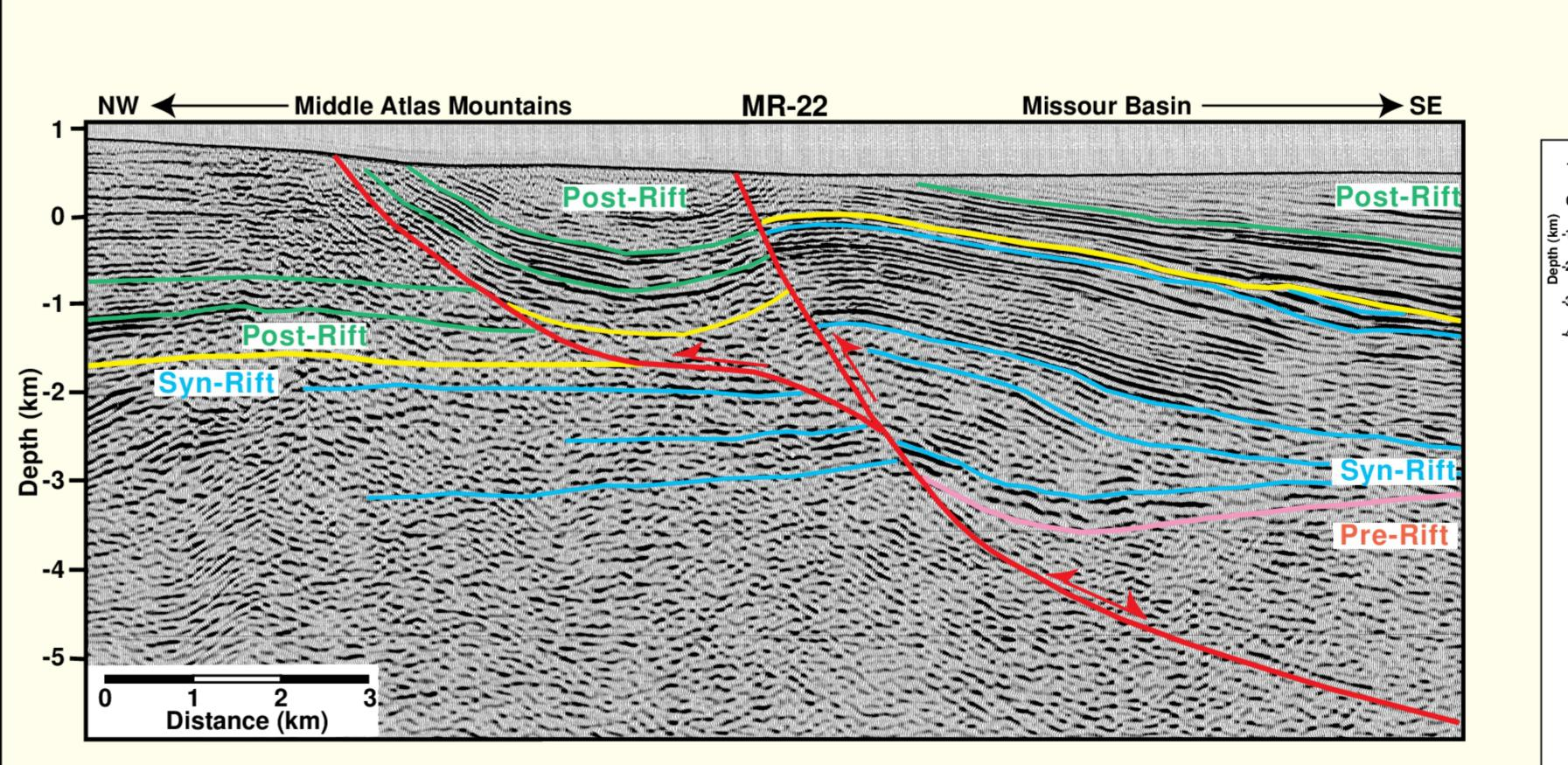
bove) Seismic line MR-22 from the southeastern margin of the Middle Atlas mountains. This line was migrated, depth converted and displayed with no vertical exaggeration to illustrate the structural geometry of a reactivated syn-rift fault and a resulting footwall short cut fault. Reflections in syn-rift age rocks show thickening into a listric normal fault.
