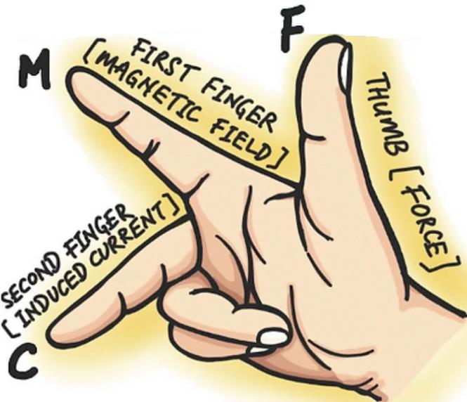
The Left Hand Rule applies to DC (direct current) motors, during times where the current and the directions of the magnetic field are known ; the Left Hand Rule gives the resultant force's direction.
