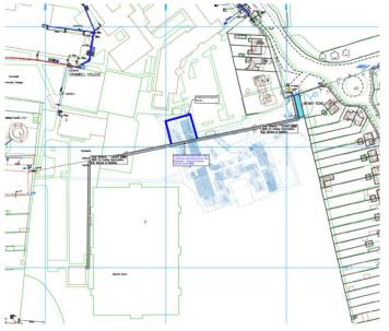
This included Granite changing the 11kV cable route to allow excavation progress around planned foundations for the new college building, which reduced the programme while allowing partial use of the college which gained them additional revenue.
