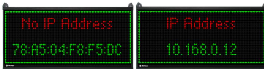
If a MAC address is displayed (left image) go to the next step: **Step 4 – Set Static IP Address.**
