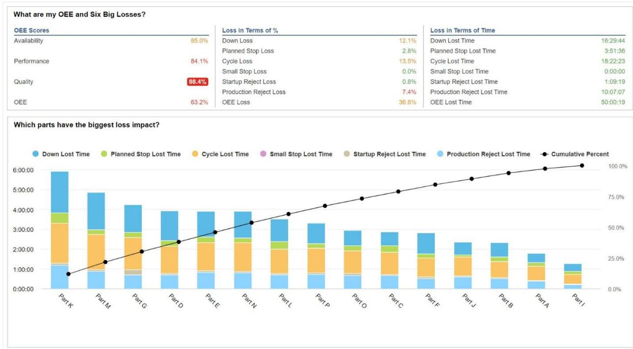
manufacturing framework that extends OEE into loss categories that each have a different set of countermeasures.
