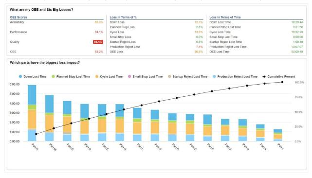
manufacturing framework that extends OEE into loss categories that each have a different set of countermeasures.
