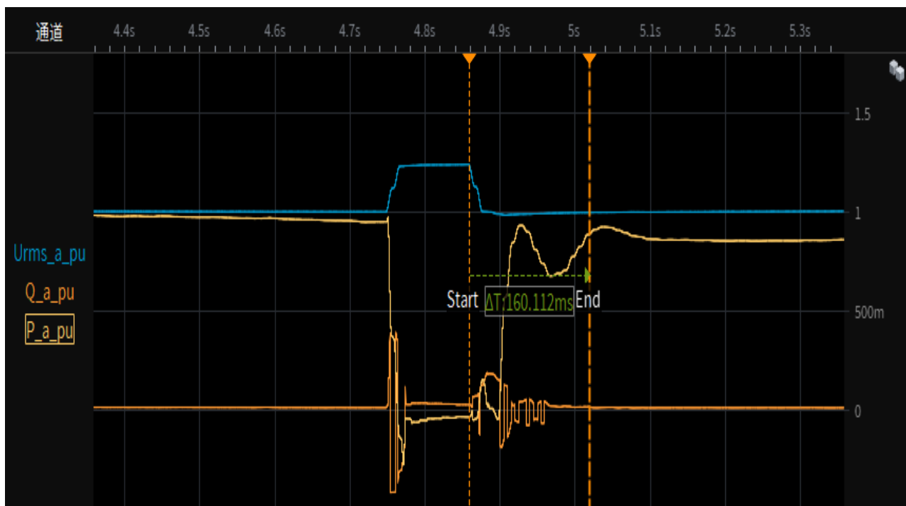
Test 8-2.4 Depth of fault phase: 1.25p.u.,three-phase-symmetrical (type A), 95% load restoring time
