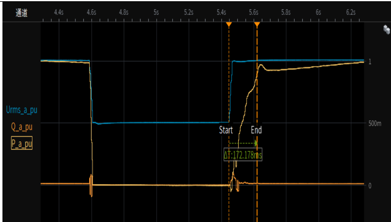
Test 3a- Depth of fault phase: 0.5p.u.,two-phase-asymmetrical (type D),0% load Test overview(voltage,current,active and reactive power)
