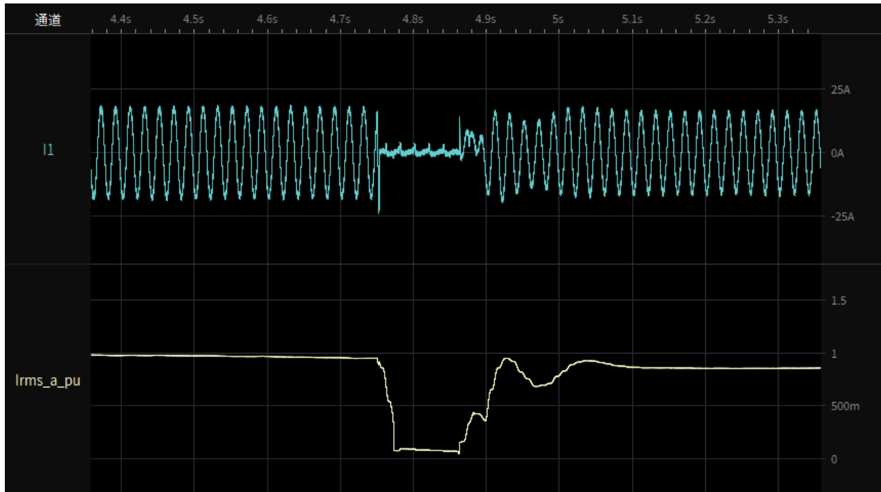
Test 8-2.4 Depth of fault phase: 1.25p.u.,three-phase-symmetrical (type A), 95% load restoring time
