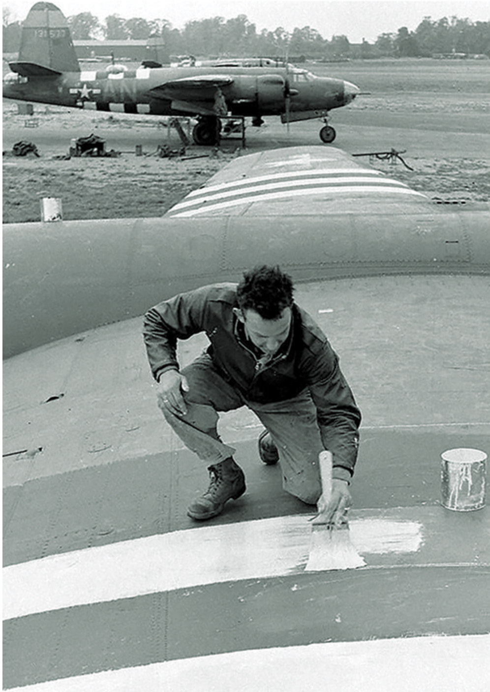
Ground crews assigned to paint aircraft in the run-up to D-Day had little trouble rendering stripes on such broad-winged bombers as these Martin B-26 Marauders. (Life Photo Collection)
