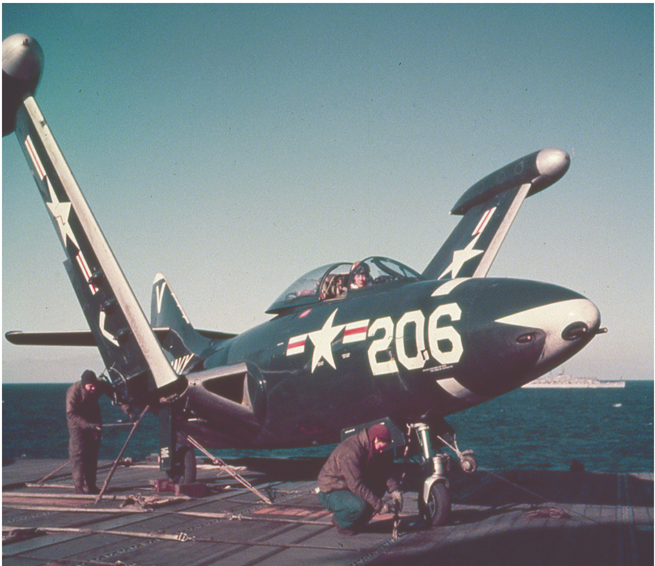
A Grumman F9F-2 Panther of fighter squadron VF-112 lowers its folding wings in preparation for takeoff from the aircraft carrier USS Philippine Sea . (National Archives)
