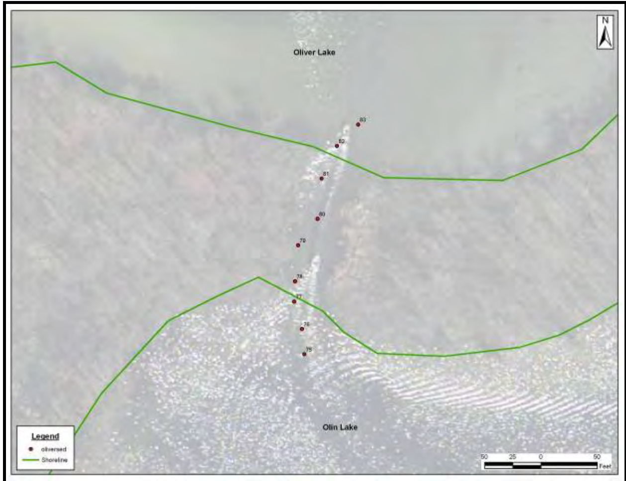
Figure 90. Distribution of sediment survey sampling points with corresponding water and sediment depths in the channel connecting Olin and Oliver Lake Site 3. Raw data can be found in Appendix I.
