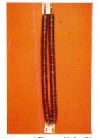
Made out of Chrome Nickel Steel tube, designed for rapid and uniform heat transfer for forced convection air heating. Ideal for use in air ducts and blower types heaters. For industrial process work, requiring heated air blast for drying, heat treating, annealing and for localised uniform heating of areas.
