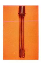
Made out of Steel tube for fuel oil heating, oil circulating, for systems which supply hot oil to plastic processes, oil jacketted kettles and similar equipment. Specially designed not to carbonize oil. Provided with thermostat pocket.
