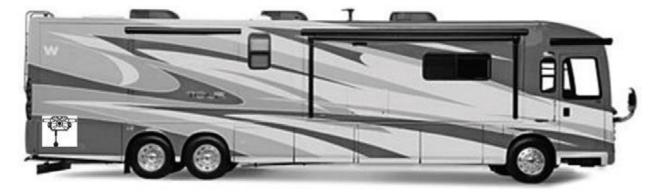
Fifth Wheel Placement: It is recommended to install the Repeater in an outside compartment under the front bed area.
