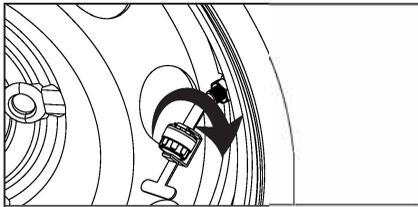
Install the sensor onto tyre valve clockwise.
