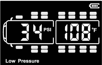
The image shows a digital monitor display with a black background. On the left, a tire icon is highlighted with a white border, and the number '34' is displayed next to 'PSI'. On the right, the number '108' is displayed next to '°F'. At the bottom left, the text 'Low Pressure' is shown. In the top right corner, there is a battery status icon consisting of four horizontal bars.                                                                          |
