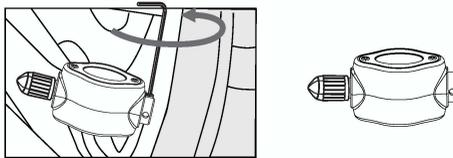
*Remove the screws from the sensor cap and remove the cap.*
