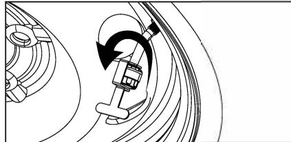
Use the spanner provided to screw the hex nut to the sensor and tighten it.
