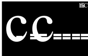
2. It will automatically move to the next window which will show you °F (Fahrenheit) or °C (Celsius) for the degree setting in the second window. Use the + or - key to scroll between the two. When the one you want to use appears in the screen press the **SET** button and release.
