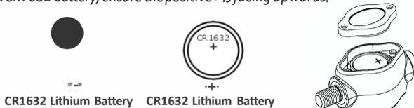
*Check that the waterproof rubber seal is in its proper position. Screw the sensor cap back on.*
