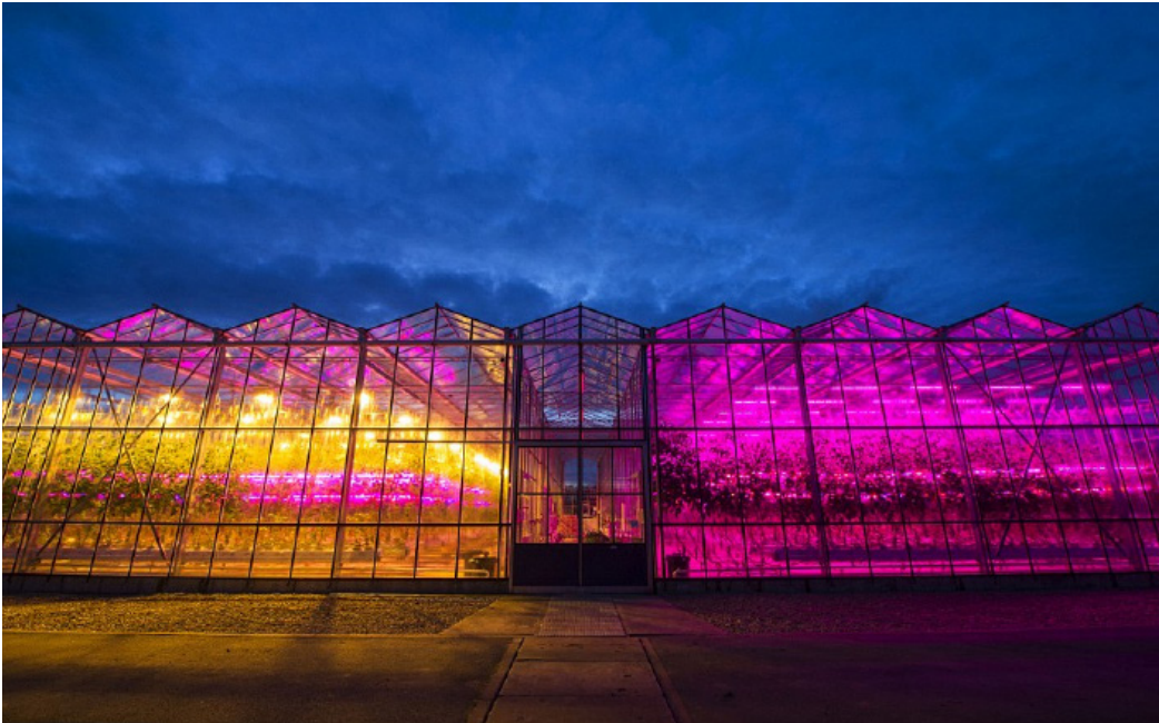
Supplemental lighting (HPS and LED) used in a glass greenhouse.
