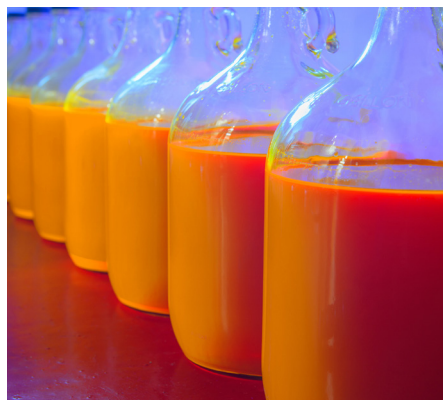
Solutions of quantum dots are prepared to make the UbiGro film.
