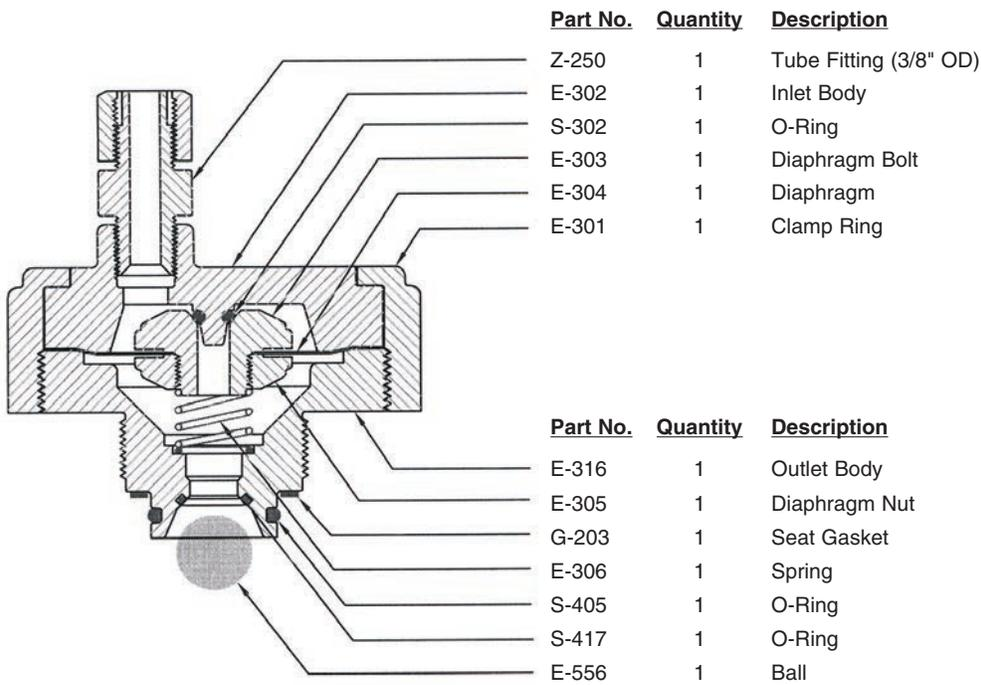
**DRAWING NO. A-950/A-949 Ejector/Dual Check Valve Assembly (Optional)**
