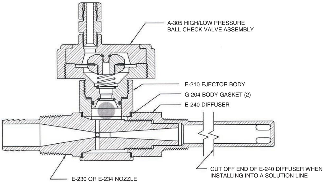
**A-305 High/Low Pressure Ball Check Valve Assembly - 100 PPD (2000 GM/HR) Maximum**
