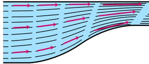
**FIGURE 16.7** Streamlines in a contracting channel. The water speeds up as the channel narrows and the velocity vectors increase in length.
