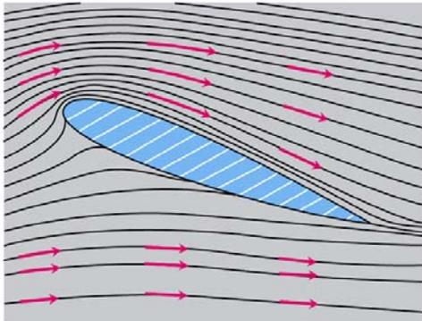
**FIGURE 16.6** Velocity vectors of a flow around an airfoil in a wind tunnel.
