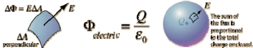
The [electric flux](#) through an area is defined as the [electric field](#) multiplied by the area of the surface projected in a plane perpendicular to the field. Gauss's Law is a general law applying to any closed surface. It is an important tool since it permits the assessment of the amount of enclosed charge by mapping the field on a surface outside the charge distribution. For geometries of sufficient symmetry, it simplifies the calculation of the electric field.
