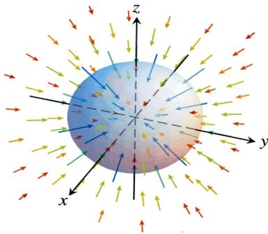
**FIGURE 16.8** Vectors in a gravitational field point toward the center of mass that gives the source of the field.
