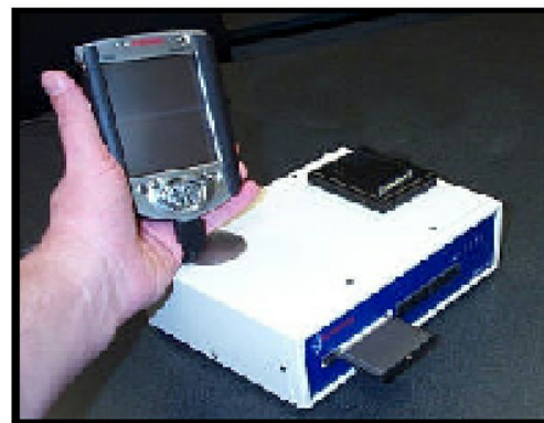
E-Tag with Equipment Simulator Clockwise: Compaq iPaq (in hand), P-Tag (black box), E-Tag (white box)
