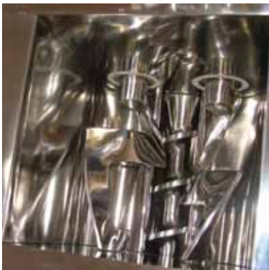
Mirrorlike polishing of contact parts
