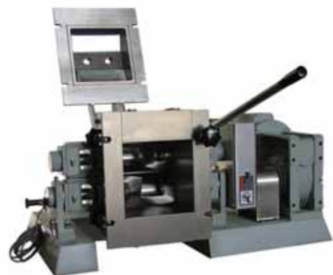
Sigma Kneader with blades working in counter-direction & tangential way
