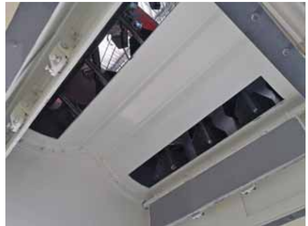
Bomb-bay door for fast & complete discharge
