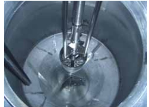
Inside view of Jet Disperser (O type) in a tank
