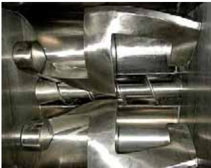
Inside view of a Sigma Kneader Extruder, with double-sigma blades and a screw extruder below for discharging
