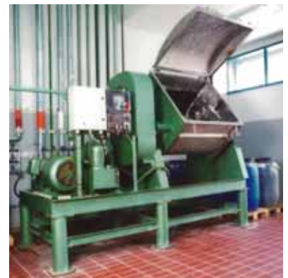
Sigma mixer by tilting discharge
