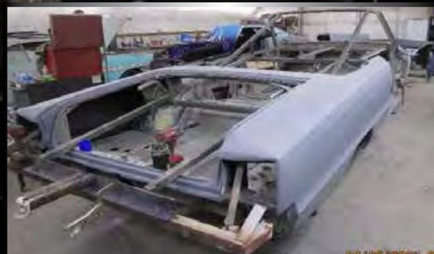
The body was very rotted in some spots, so care was taken to keep the body aligned on a jig until the structural work was completed. The cage had to be removed to install the replacement panels and re-installed in sections once that part of the work was completed. Work stopped for a few months as IVR worked on finishing cars for the Feb 2020 World of Wheels and the holiday season came up.
