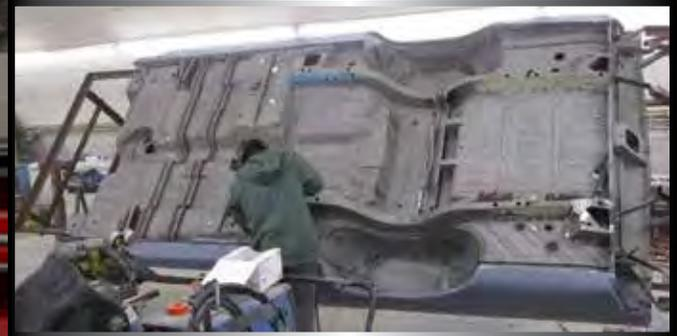
A mint condition floor was transplanted from a parts car. A rust free replacement trunk floor and wheel well assembly was removed from a parts car and transplanted to the convertible. The best quarter panels of all were removed and welded onto the convertible body.
