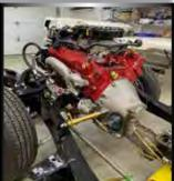
On December 18, Dean Tilleman came over to Terry's shop to lead the engine start up. After figuring out the final wiring connections, the Monaco was fired up for the first time in over 30 years. There was a knocking that had to be diagnosed. Terry figured out the noise was coming from the release bearing and fixed it, so the big block ran well.
