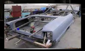
The body was very rotted in some spots, so care was taken to keep the body aligned on a jig until the structural work was completed. The cage had to be removed to install the replacement panels and re-installed in sections once that part of the work was completed. Work stopped for a few months as IVR worked on finishing cars for the Feb 2020 World of Wheels and the holiday season came up.
