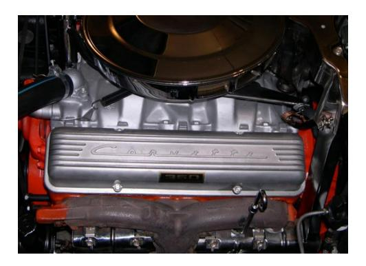
Notice that aluminum paint appears on the water pump bypass hose. The inboard edges of the heads should also exhibit an aluminum painted surface. The sheen should be a flat finish. I typically use a high-temperature, flat aluminum paint.
