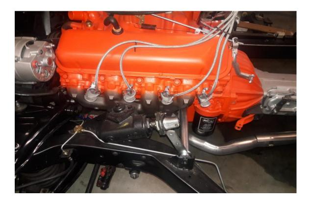
Notice that I applied orange paint only to a small part of the upper exhaust manifolds since that is where the paint tends to remain after engine run. The factory certainly painted the exhaust manifolds more liberally, but as I mentioned before, why would I want hot orange paint embers to fall on my black frame?
