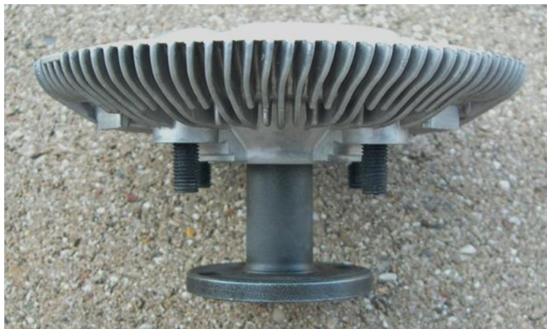
Eaton-style fan clutch straight shaft Figure 3
