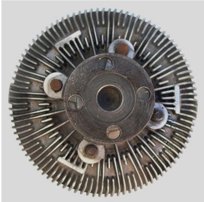
Eaton-style fan clutch back Figure 2
