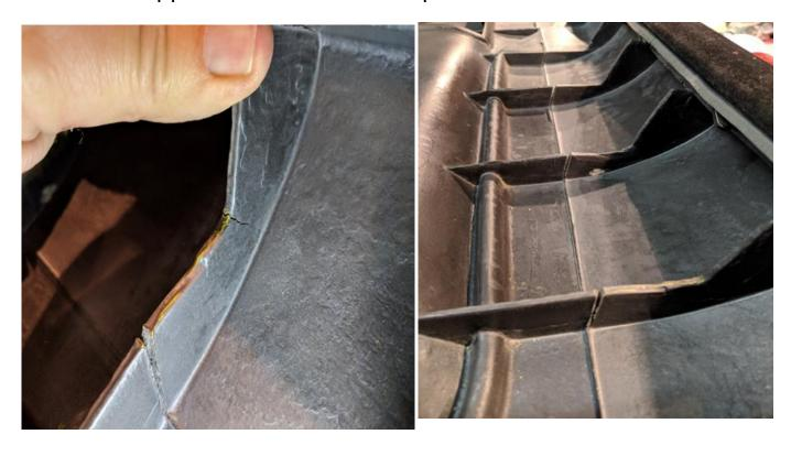
"ribs" cracked, the door panel flexed enough to allow the top to disengage from the door frame structure. The door panel could be reengaged with the door frame only to pop off when shutting the door.
