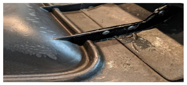
On the passenger's door panel I used flat plastic strips that I cut to fit and epoxied to the ribs.
