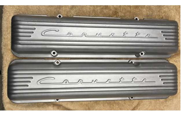
Sometime in 1966, the die-casting mold was damaged and repaired. The repair would leave a casting flaw mark across the cover running through the letter "o" in the "Corvette" script. This valve cover should be considered as not factory correct for a C1 Corvette. Correct valve covers should be the right configuration for the car. They should not be polished or coated or painted.
