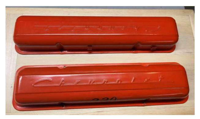
Another big distinction between valve covers is the alignment of the bolt holes that attach the cover to the cylinder head. Early cars have staggered bolt holes but in late 1959 production, Chevrolet aligned the holes to straight across. Thus these covers are often referred to as <u>staggered</u> or <u>straight aligned</u> valve covers.
