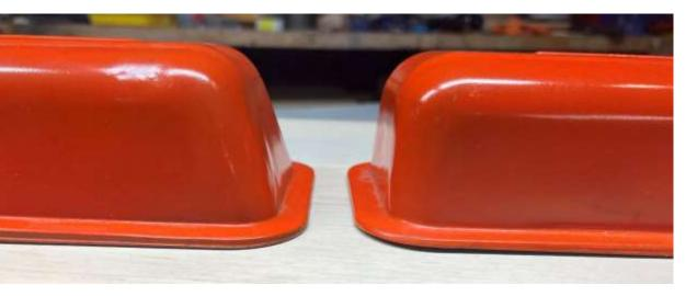
The first cast aluminum covers were introduced in 1956 and used through the 1957 model year. The raw aluminum casting has a somewhat dull finish and may show some spots of discoloration or minor casting flaws. They have nine longitudinal ribs.
