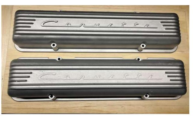
But Chevy wasn't done yet. In late June of 1959, they changed to the straight aligned bolt hole heads and valve covers. This valve cover became the standard cover from 1960 through 1967.
