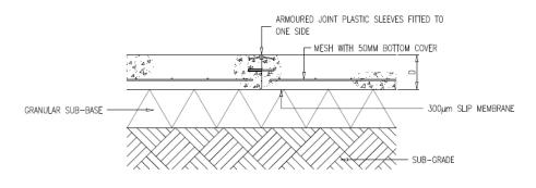
Figure 1: Typical armoured construction joint detail
