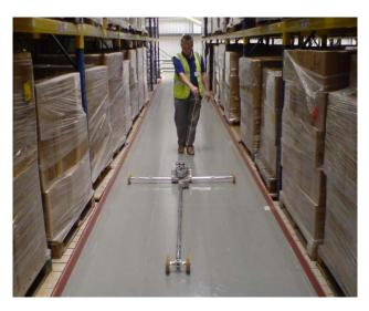
Figure 7: Face Digital Profileograph within a narrow aisle
