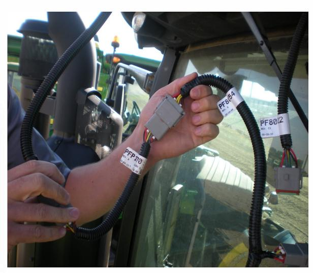
Connect the PF10470 to the Speed and GPS cable PF80754
