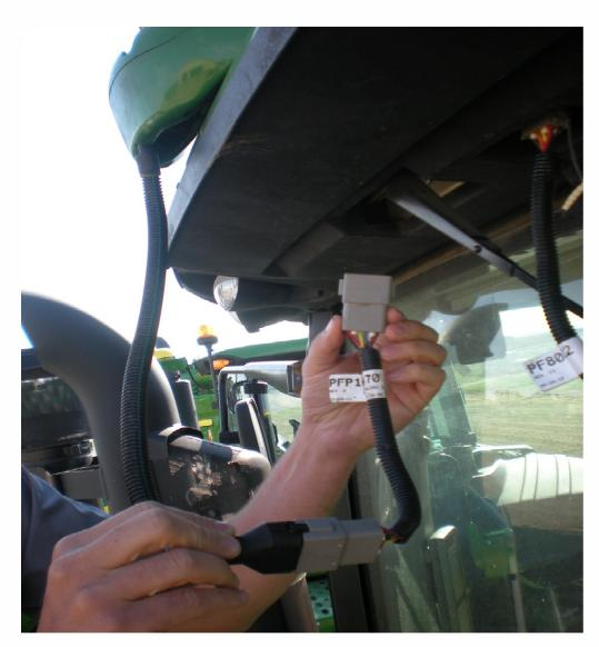
Connect the female/female PF10470 to the receiver cable that was unhooked from the tractor earlier.
