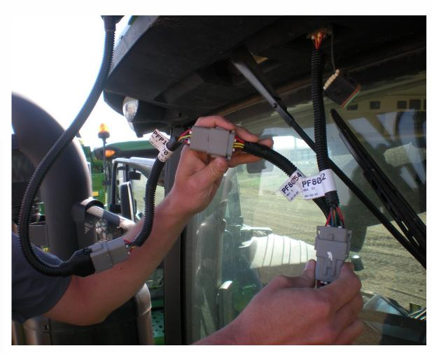
Connect the PF80722 to the Speed and GPS cable PF80754
