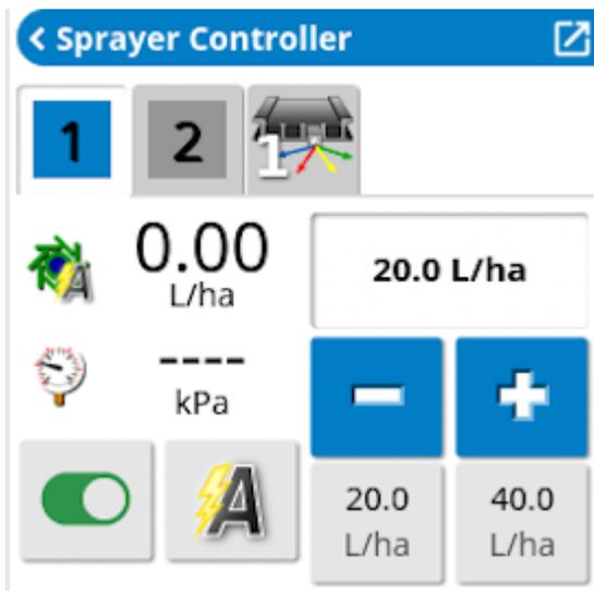
The icon at the top of the mini-view is the same for all tank types but the displayed units change (nitrogen amount per area for NH<sub>3</sub> and a fraction of the liquid tank unit for the chemical injection tank). Displayed units may be changed via **User / Region / Units**.
