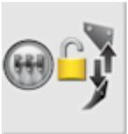
Drill lift/lower track master (control down force using the master switch)
