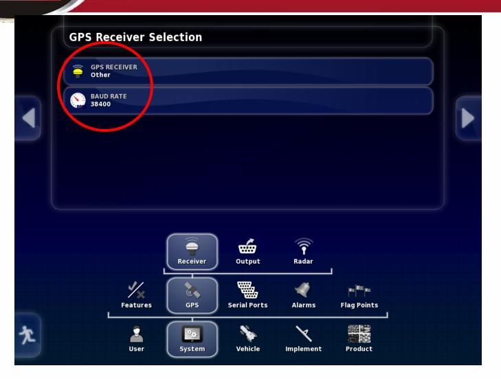
Set GPS RECEIVER to Other and the BAUD RATE to match the John Deere output rate
