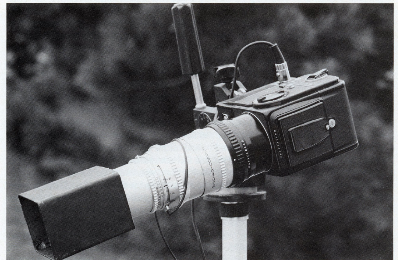
Jeklin's Hasselblad 6 cm × 6 cm EL/M (electric motor drive) equipped with the 55 mm extension tube and the 5.6/250 mm Sonnar lens.
