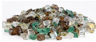
The Tumbled Glass Sand was then used to make concrete retaining wall blocks. The Tumbled Glass Gravel was blended 50/50 with the glass trim paste to produce high quality recycled-content construction aggregates. The aggregates have been used in various construction projects across Massachusetts.
