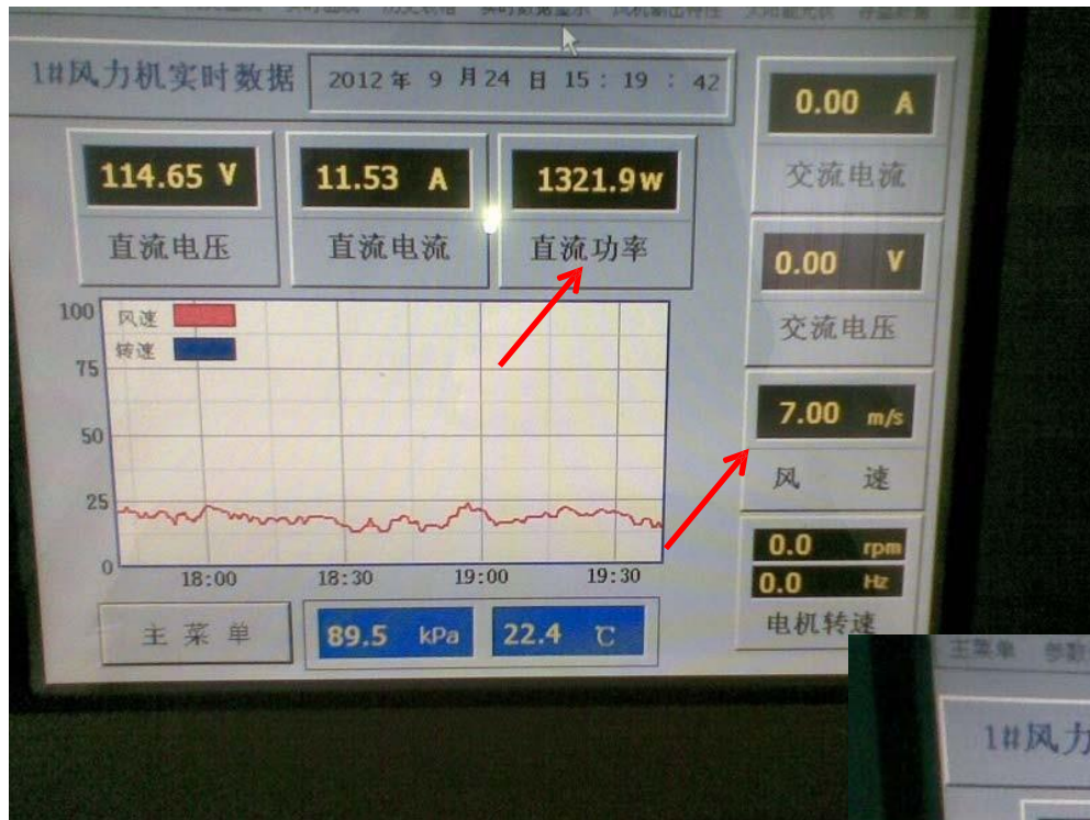
P.10 Real Time Data of Turbine No.1
