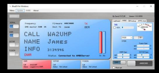
BlueDV supports DMR, Dstar and soon to support Fusion. It can run under Windows, Linux, IOS and Android. To run as a hotspot you need a DVMega radio/modem board. The DVMega sits on a Bluestack board or an Arduino. DVMega boards are costly. The Dual Band board is about \$170. Bluestack is about \$70. Assembled DVMega with Bluestack and case is about \$260. Web Site: http://www.pa7lim.nl/bluedv-windows/
