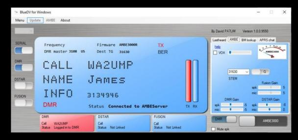
BlueDV also supports an AMBE Vocoder such as the ThumbDV. It cost about \$120. With the vocoder BlueDV does not operate like a hotspot. It operates like a network radio. You use your computer speakers and mic and operate as if it was a radio. No RF is used. In this mode your ham transceivers do not interact with BlueDV. However, if you have Your radios on a repeater or hotspot on the same talk group as your BlueDV they can hear each other.
