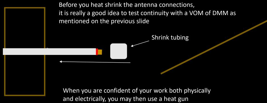
or lighter to carefully "shrink" the tubing over the connections!
