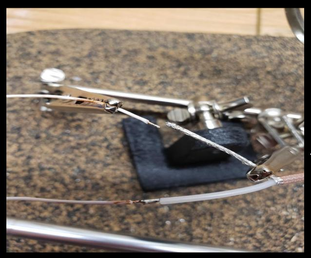
After stripping about 2-4mm of the coaxial cable center conductor, solder one length of the wire coming out of the bottom of the pen body.
