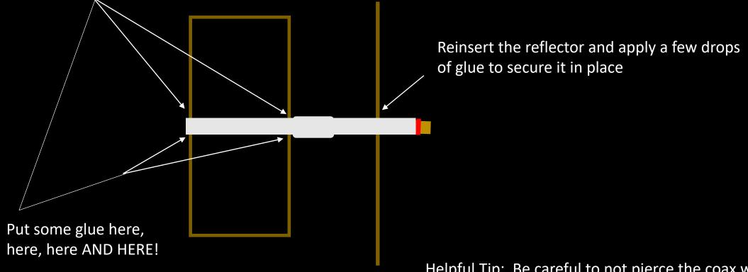
Helpful Tip: Be careful to not pierce the coax when sliding the reflector into the antenna pen
