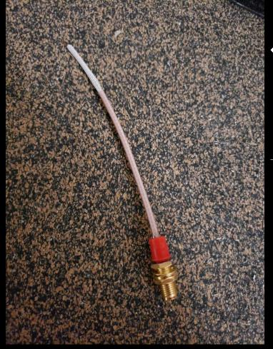
Properly completed matching section with the outer jacket of the RG-179 coaxial cable stripped at 57.6mm
