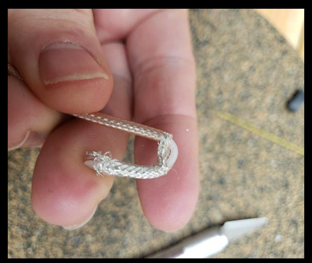
Once you can get to this stage, it should be easy to pull the rest of the center conductor through the braiding. Do not be tempted to unbraid the shield as an alternative method of separating the coax as it will make a mess and complete antenna assembly.
